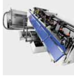
The V-shaped conveyor belt ensures gentle labeling of round or odd-shaped products
