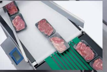
The Bizerba LCE line converger optimises package handling in material flow systems. By taking multi-lanes (1 to 6 lanes) of packed products and converging them into a single line, it enables the reliable and controlled transport of goods from packaging machines to price labellers (Bizerba GLM-I and GLM-E) and checkweighers (Bizerba CWE). The LCE has proven itself to be a highly flexible, efficient and fail-safe solution in almost all industry sectors.
