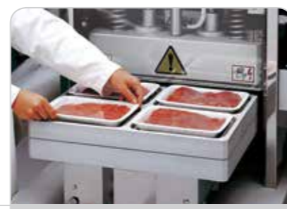
Tray Ejection with Adjustable Up Time
