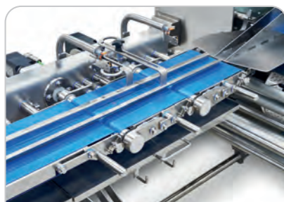
"Open Frame" design washdown and Sanitary design infeed conveyor
