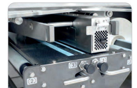
"Easy-Tape" system to facilitate the automatic reel splicing
